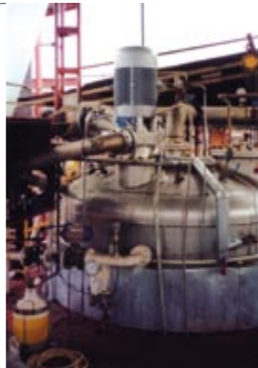
Defoamer 600P mounted on production-fermenter for biopolymers
