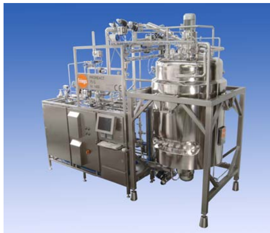
Figure 2: FRINGS PROREACT 75 with foam centrifuge FOAMEX on top
